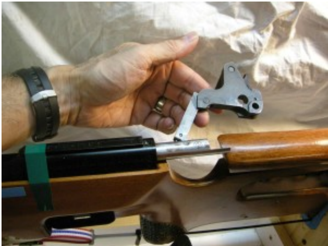
4) remove bolt sliding it out in a rearward direction.
