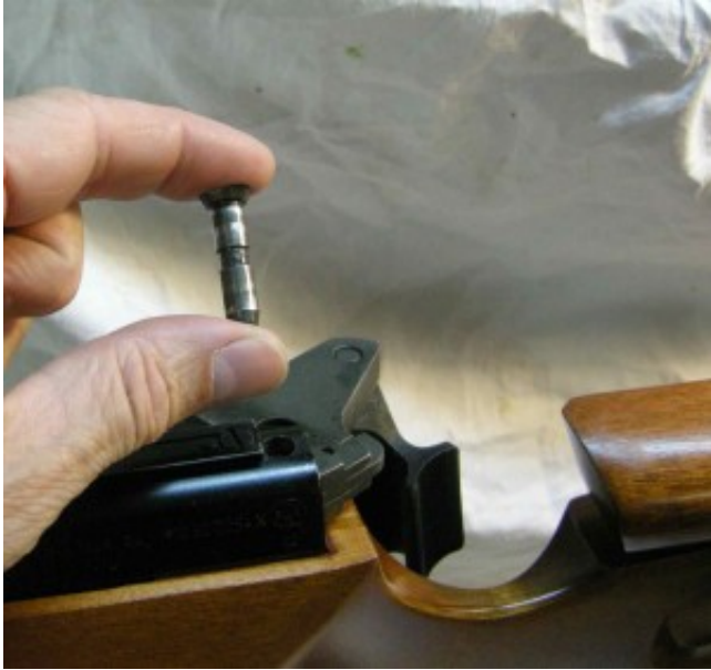
4) remove bolt sliding it out in a rearward direction.
